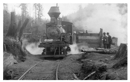
Another type of logging locomotive common in the Northwest was the Climax, characterized by two cylinders, mounted at an angle fore-and-aft, one on each side of the engine. Sobey Mfg Co., later Waite Mill, operated a Climax locomotive, shown here being refueled near the mill.
